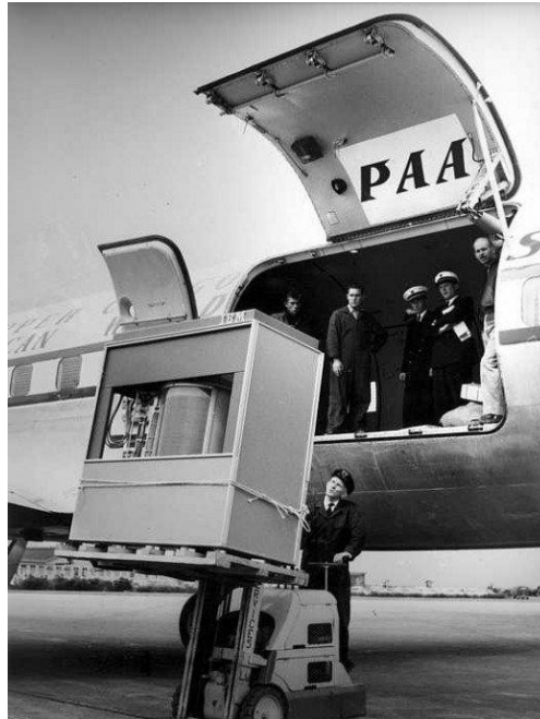
1956: A 5 megabyte IBM harddisk is loaded into an airplane. It weighed over a 1000kg
